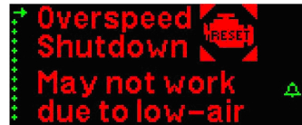
Engine Over-Speed Shutdown Low Air Warning
