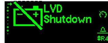
Low Voltage Disconnect
