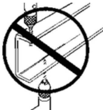
FIGURE 4-8. Frame Rail Flange Drilling Prohibited
