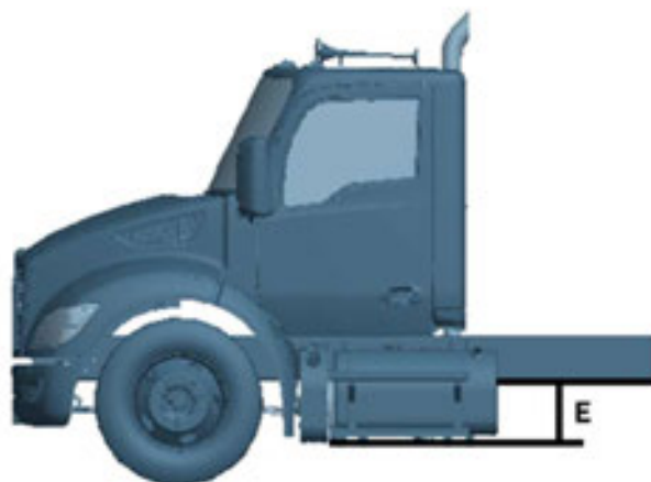
FIGURE 3-12. Bottom of Frame to Bottom of Component
