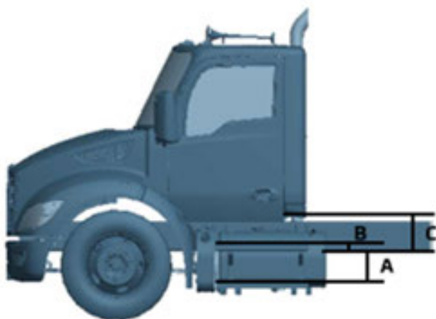
FIGURE 3-9. Cab Step Height Dimensions (Table 3-2)
