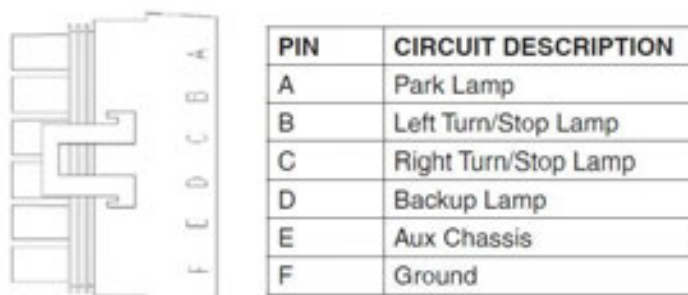
FIGURE 7-38. 6-Way Tail Light Connector Pinout
