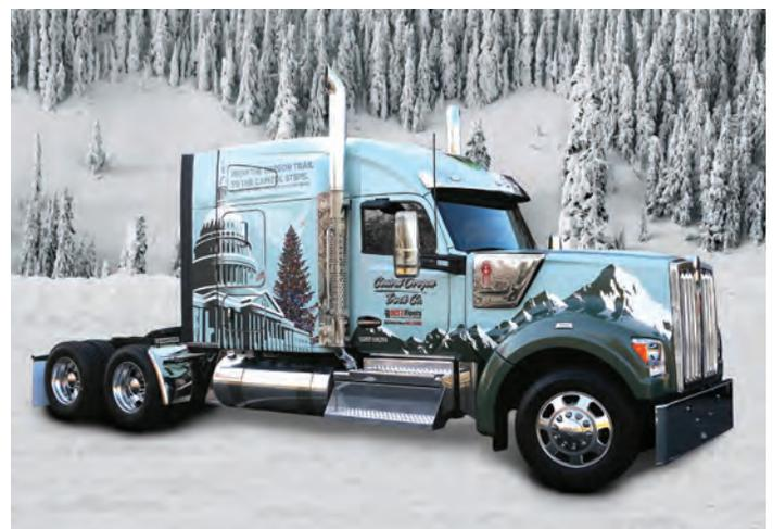
*The new Kenworth W990 will transport the 2018 U.S. Capitol Christmas Tree from Oregon's Willamette Forest to Washington, D.C. The W990 is equipped with a 76-inch-mid-roof sleeper and the proprietary powertrain of PACCAR's MX-13 engine, 12-speed automated transmission, and 40K tandem rear axle. Central Oregon Truck Company in Redmond, Ore., was selected as this year's tour hauler. In commemoration of the Oregon Trail's 175th anniversary, the route will follow a reverse path of the famed trail.*
