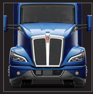
The front bumper design and air dam increases air flow under and around the truck while maintaining ground clearance.
