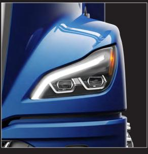
Optional LED headlamps with built in heaters increase down-road vision in inclement weather and improve night time viability.
