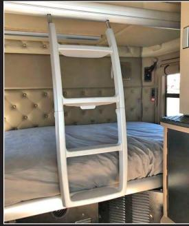
Optional upper bunk ladder folds away when not in use. This provides an alternative way for drivers to access the upper bunk.
