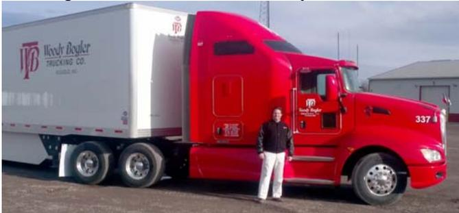
*Tracy Bogler, president of Woody Bogler Trucking, is shown with one of the company’s fuel-efficient Kenworth T660s equipped with the PACCAR MX engine.*
