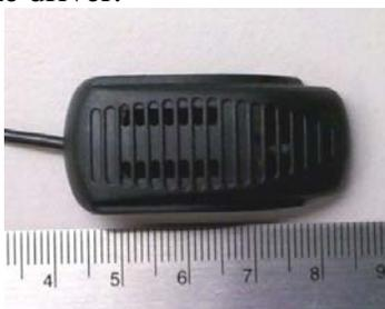
*A small Bluetooth microphone is mounted on the A-pillar trim above the driver.*
