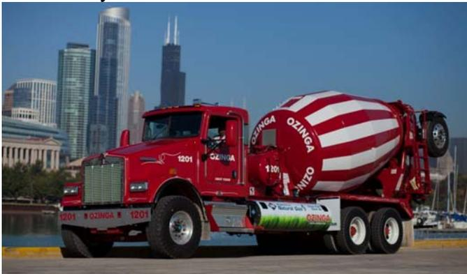
Leading the way is the Kenworth W900S natural gas mixer, which is equipped with the Cummins Westport 8.9-liter ISL G engine, Allison 4500RDS 6-speed automatic transmission and McNeilus Bridgemaster mixer body. Rated at 320 hp and 1,000 lb-ft of torque, the ISL G uses a maintenance-free, three-way catalyst and is 2010 EPA and CARB compliant without the use of selective catalytic reduction (SCR) technology or a diesel particulate filter (DPF).
