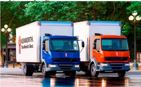
Kenworth K270 and K370 applications include pick-up and delivery, lease/rental, towing/recovery, landscaping, furniture, and food processing and distribution that require a highly maneuverable truck with 18- to 26-foot van body size, stake bed, or roll-on/roll-off bed. The 63.4-inch BBC (front bumper to back of the cab) on the K270 and K370 provides a 55-degree wheel cut.
