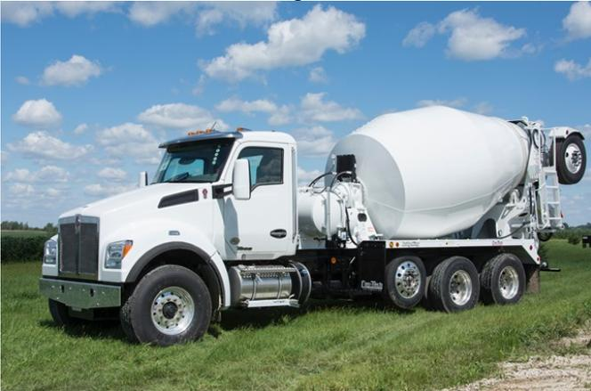
The T880S with a set-forward front axle is equipped with a PACCAR MX-11 engine rated at 430-hp and 1,650 lb-ft of torque, and a BridgeKing® 11-cubic yard bridge formula mixer with a high performance drum contributed by Con-Tech Manufacturing.
