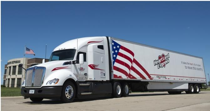
The fleet’s new model Kenworth T680 76-inch high-roof and mid-roof sleepers, powered by PACCAR MX-13 engines, provide superior performance, reliability and driver satisfaction. During a special ceremony last year, Gerdin rewarded his top drivers with the keys to the company’s first, newly-delivered 2017 Kenworth T680s, demonstrating Heartland’s highest regard for the quality and comfort of Kenworth.
