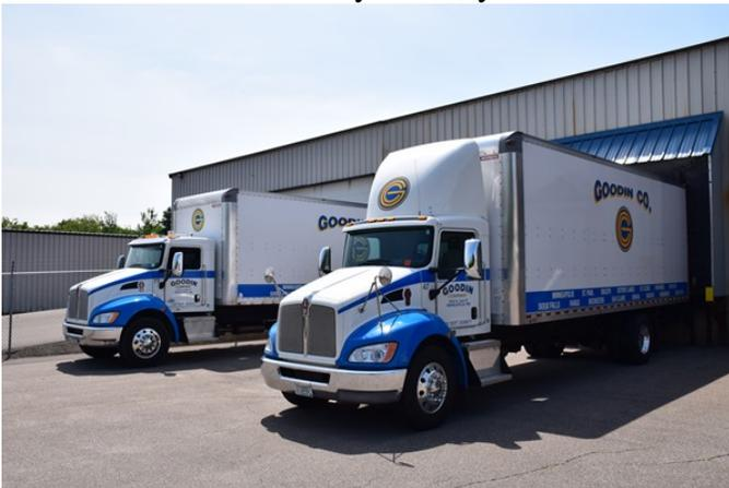
New trucks are spec'd with the PACCAR PX-7 engine, rated at 300 hp, and driven through Allison automatic transmissions. Drivers appreciate the comfortable ride, excellent visibility, easy handling and rugged dependability in all weather conditions.
