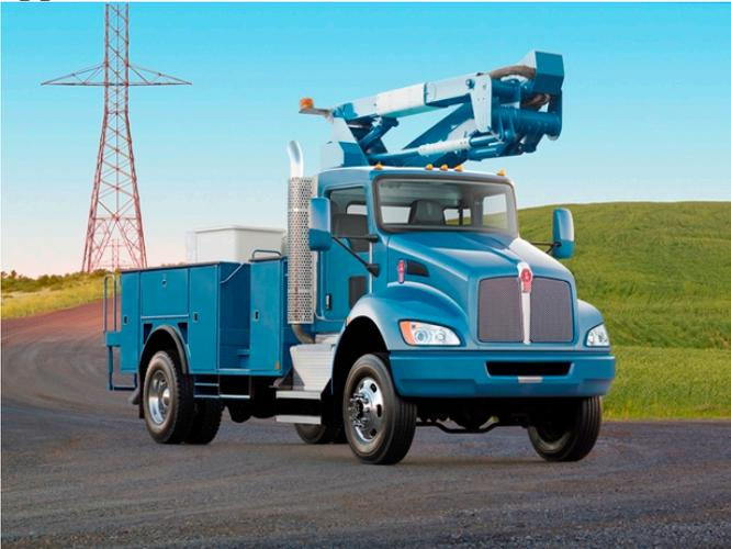
The Kenworth T370 offers the Fabco FSD-18A and FSD-20A front drive axles paired with an all-new Fabco TC-548 transfer case for exceptional durability. The two front drive axles are available with the PACCAR PX-9 engine rated up to 350 hp and 1,150 lb-ft of torque. Both models require taperleaf front springs, and are available with air or mechanical rear suspensions.
