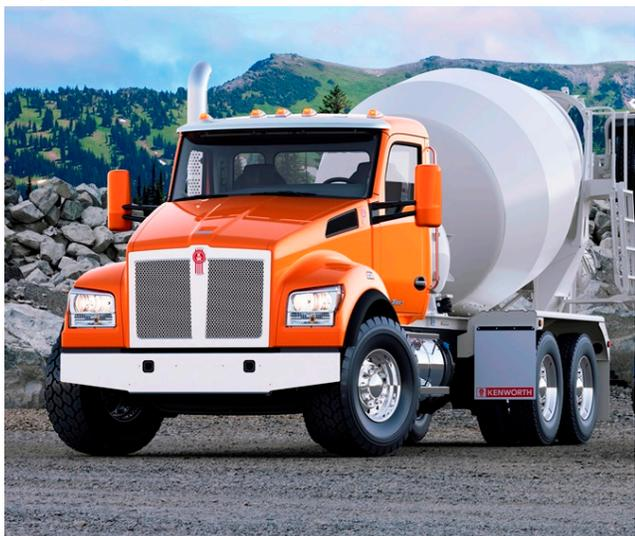
The T880S is offered with a set-forward front axle ranging from 14,600 pounds to 22,800 pounds, and is standard with the PACCAR MX-13 engine with up to 510-hp and 1,850 lb-ft of torque. For weight-sensitive applications, the 10.8-liter PACCAR MX-11 engine is 400 pounds lighter compared to larger displacement engines, and provides up to 430-hp and 1,650 lb-ft of torque.
