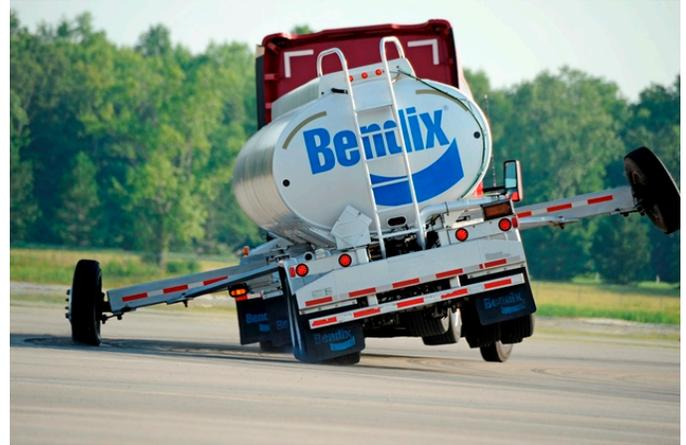
*The photo shows a vehicle on a demonstration track where the stability system is turned off. The outriggers are installed during demonstrations to keep the vehicle from rolling over.*
