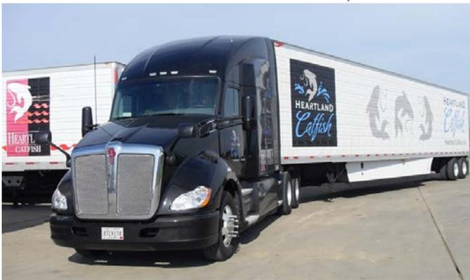
With a fleet of 22 Kenworth T680s, Itta Bena, Miss.-based Heartland Catfish has converted its fleet of high-hood trucks into a fleet of T680s that are not only making drivers smile, but accountants as well. The aero model has gained the company 2.3 in mpg over its previous long-nose, which means a fuel savings of more than \$2,000, per truck, per month. That’s more than a \$44,000 monthly cut in the cost of fuel for the fleet.
