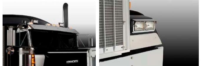
Other distinguishing features include stainless steel fender guards, upgraded headlights, headlamp covers, under door panels and sleeper panels, grille closeout panel, plus large sun visor are just some of the items that create a stunning exterior package. The Kenworth ICON 900 is available with 72- or 86-inch sleepers and up to a 600-hp engine.
