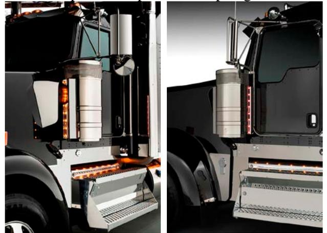
"LED panel lights mounted under the cab and sleeper panels, along the roof, and to the front and rear of the stainless air cleaners make the truck visually spectacular when running at night," said Skoog. Amber LED side turn indicators and 4-inch sealed LED stop, turn and taillights emit a unique glow for a special ambiance.
