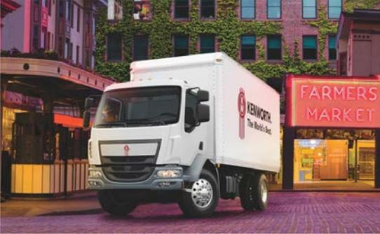
The new options for the Kenworth K270 and K370 cabovers include a compact back-of-cab exhaust system to allow more space for custom bodies; right-side steer for street sweeping, refuse and road maintenance applications; and expanded PACCAR PX-7 engine ratings.
