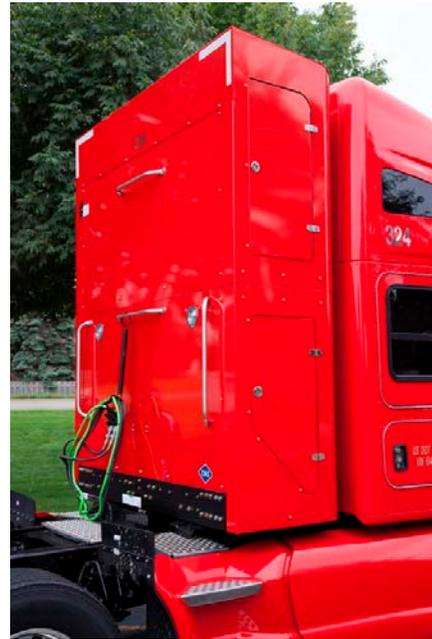
Paper Transport has equipped its Kenworth T680 with 76-inch sleeper with Agility Fuel System’s new 155-gallon diesel gallon equivalent behind-the-cab compressed natural gas (CNG) fuel system. The Agility system utilizes four 26-inch by 80-inch Hexagon-Lincoln Type 4 cylinders, weighs only 2,550 pounds and requires only 31.25 inches of frame rail space. It can deliver a range of about 600 miles before refueling, which offers the industry’s best DGE per inch of frame rail.
