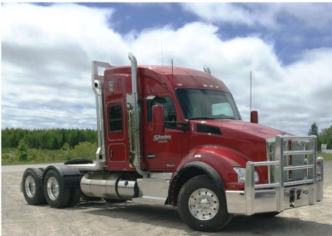
*S Nychuk Excavating operates a new Kenworth T880 52-inch sleeper with a 500-hp PACCAR MX-13 engine.*
