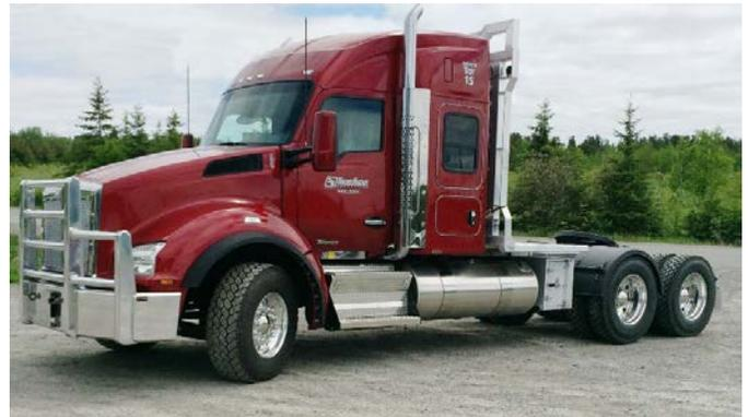
"We need trucks equipped for a variety of on-highway and off-highway hauling," said Nychuk. The company recently took delivery of its first Kenworth T880, equipped with air suspension, a 52-inch sleeper, a 500-hp PACCAR MX-13 engine and an 18-speed transmission. The T880 is assigned to his father-in-law, Carson Presseault.
