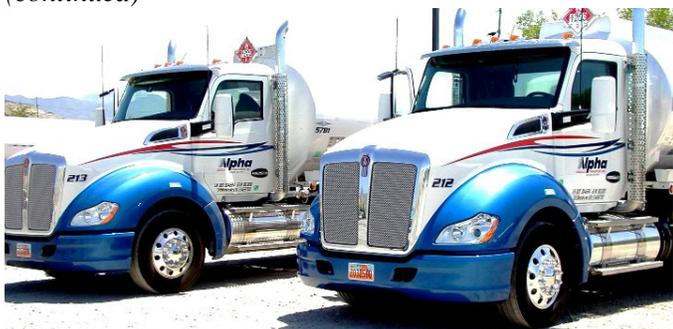
Hauling 110,000 pounds GCW (gross combination weight) for a typical fuel delivery, the Alpha Transport's Kenworth T680 day cabs with 249-inch wheelbase support a tanker that typically carries 5,200 gallons, while also pulling a tanker normally filled with 6,800 gallons.
