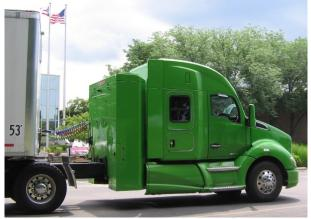
Kenworth displayed a T680 52-inch sleeper equipped with the Cummins Westport ISX12 G engine powered by CNG at this year's Mid-America Trucking Show and at the annual Alternative Clean Transportation (ACT) Expo. Kenworth also offers the ISX12 G in the Kenworth T660 and the Kenworth T800 short hood with a 116.5-inch BBC.
