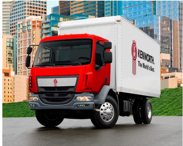
“Compared to a typical medium duty conventional, the K270 and K370 offer up to a 30 percent better curb-to-curb turning radius, a 63.4-inch BBC with an extra 45 inches of payload room, and a 35-foot overall length which is rapidly becoming the new norm in major cities,” Powell said.
