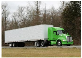
Key weight-reducing components are the 12.9-liter PACCAR MX-13 engine, Eaton Fuller Advantage<sup>TM</sup> series transmission, Kenworth AG380 suspension, MX optimized hood (119-inch BBC), 6x2 drive axle, rear wide-base single tires, aluminum rear wheels, air disc brakes, and aluminum fifth wheel.
