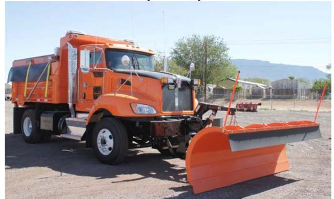
Bigger than a Class 7 truck and smaller than a Class 8, the T470 is available in GVW ratings from 33,000 to 68,000 pounds. The New Mexico DOT spec'd 14,600-pound front axles (ratings are available from 12,000 to 22,000 pounds), and rear axles at 23,000 pounds (single rear axles are available from 21,000 to 30,000 pounds, and tandem rear axles from 40,000 to 46,000 pounds).
