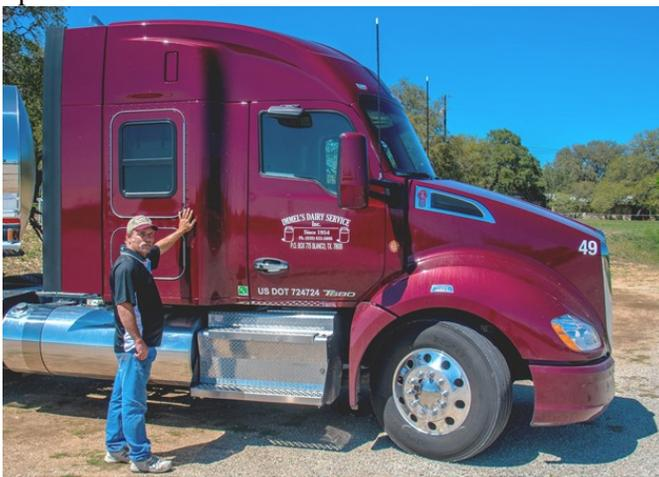
Since Immel’s Dairy Service picks up loads at dairies, the mid-roof 52-inch sleeper was spec’d. “This lowers our profile so we can slide under loading areas without fear of hitting the overhead structures,” Immel said. “Our guys will be out six days at a time, so they use the sleeper. The height, compared to the height of our other sleeper, is what I really like.”
