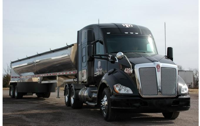
With 16 new T680 mid-roof sleepers operating in the fleet, Bogler said some of the new Kenworth trucks are getting over 8 mpg, with an average of 6.8 mpg across the entire fleet of 142 trucks.
