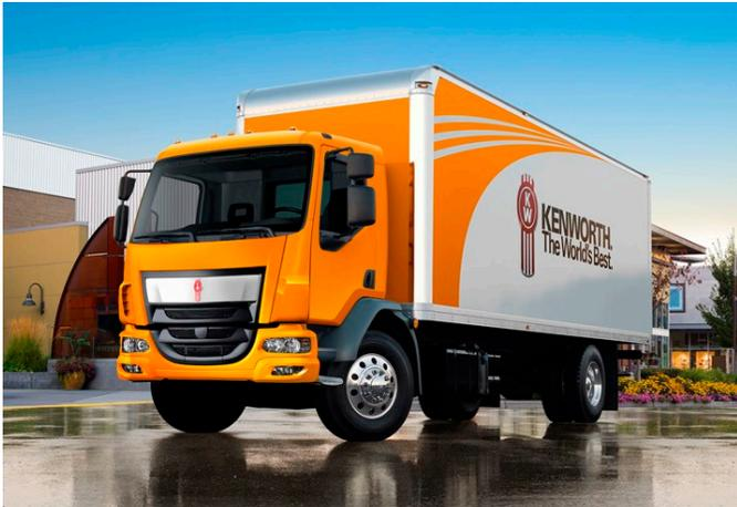
Available with wheelbases ranging from 142 to 242 inches in 12-inch increments, the K270 and K370 can accommodate bodies from 16 to 28 feet. A large 2,500-square-inch wraparound windshield combines with large side windows to give optimum visibility.
