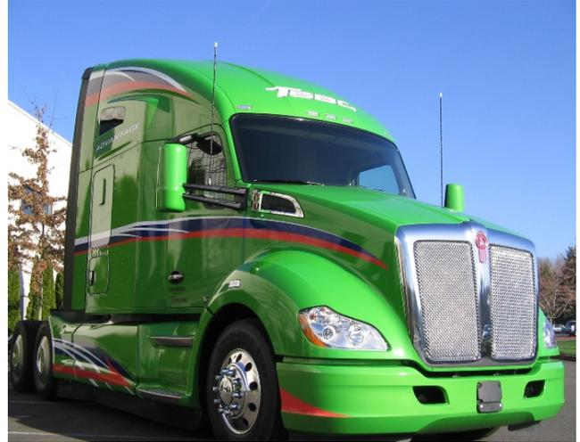
The Kenworth T680 Advantage – Kenworth’s new, most fuel-efficient truck – features a special factory-installed aerodynamic package along with the optimized powertrain combination of the PACCAR MX-13 engine integrated with the Eaton Fuller Advantage™ 10-speed automated transmission.
