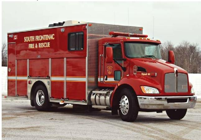
As for equipment, the five fire rescue vehicles include two Kenworth T370s with another recently purchased and awaiting a custom body. The single-axle rescue vehicles are built with 18-foot van bodies with rear walk-in. Heavy hydraulics power a 'jaws of life' life-saving cutter, and tower lighting extends 10 feet above the rescue unit. "Those are our go-to vehicles for accident response and any water rescues," said Chesebrough.
