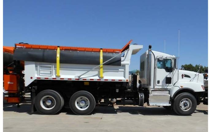
The T470s, in single-and-tandem axle configurations, serve various functions for the city. The tandem-axle units, with 10-yard dump bodies follow the city street sweepers and collect two-to-three yards of street debris in each cycle. They also haul aggregate, sand and asphalt for concrete work and crack maintenance, plus road patching jobs. The single-axle T470s are outfitted with five-yard dump bodies for lighter duty work.
