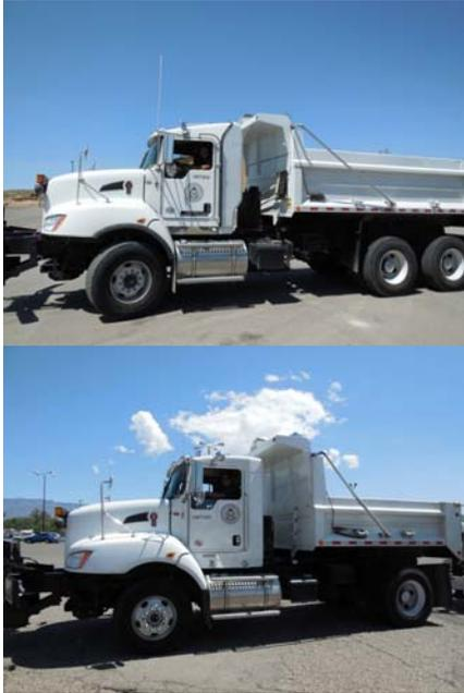
The single axle Kenworth T470s are powered by the PACCAR PX-8 engine, rated at 330 hp, while the tandems feature Cummins ISL engines rated at 380 hp. Both are driven through Allison automatic transmissions. The new T470 on order will feature the 2013 PACCAR PX-9 engine rated at 330 hp.
