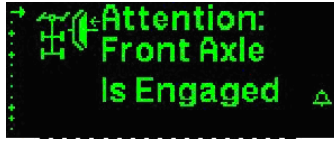
Front Drive Axle Speed Warning
