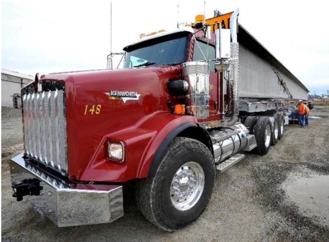
But, it's the 205-foot girders that made the project so challenging, said Bates. "We had to develop a new trailer system to handle not so much the length, but the weight," he said. All told a front trailer, with 18 wheels, connected to the fifth-wheel and cradled the front of the girder while a rear, driveable trailer with 32 wheels maneuvered the back of the load. The back was maneuvered by a driver in the cockpit of the trailer, which looked akin to a vehicle out of a Mad Max movie.
