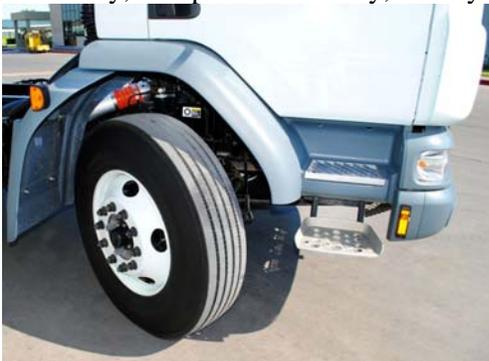
With Kenworth’s new 22.5-inch tire and wheel package, the K270 Class 6 and K370 Class 7 cabovers match up to standard dock heights at pickup and delivery locations in several applications, Powell noted. Depending on van body installation practices, the cab floor will be at approximately 50 inches up from the ground with an 11R22.5-inch package. The K270 will also retain the 19.5-inch tire and wheel package as an alternative for customers that require a lower-step height and entry.
