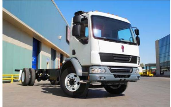
According to Powell, the new longer wheelbase allows for up to a 28-foot van body installation, while the shorter wheelbase can accommodate a van body length down to 16 feet. The cab-to-axle dimension now starts at 120 inches with variations up to 217 inches at a 242-inch wheelbase. The K270 with 19-1/2-inch tires and wheels receives four new wheelbase sizes, covering a range of 142 inches to 238 inches, also in 12-inch increments.
