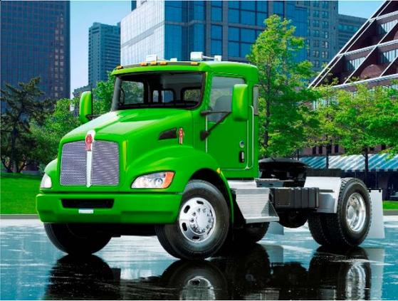
Lastly, Kenworth will show a Kenworth T370 diesel-electric hybrid, which helps to enhance fuel economy by up to 30 percent in pickup and delivery applications and up to 50 percent in utility and service operations. Hybrids are especially of interest to fleets running local routes with a significant number of starts and stops, and to municipalities seeking to save on fuel and reduce their carbon footprint.
