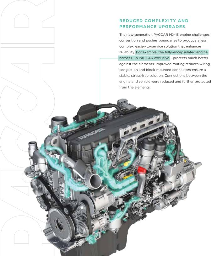
The new combined engine and aftertreatment control module eliminates wiring harnesses and connectors for a streamlined, highly-reliable design. A constant power source improves the shut-down sequence and enables immediate battery disconnect.
