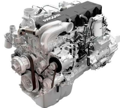
The PACCAR MX engine is available with a horsepower range of 380 hp to 485 hp and torque up to 1,750 lb-ft on selected Kenworth Class 8 models. It is an ideal choice for Kenworth customers operating in many over-the-road, pickup and delivery, and vocational applications.
