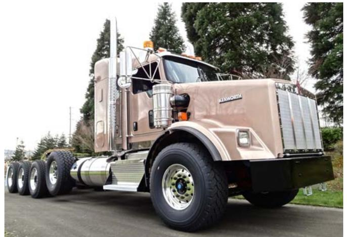
With that, Trican closed its initial truck order with GreatWest Kenworth for W900s and T800s. Over the years, the T800 became Trican’s truck of choice for its excellent versatility, reliability and maneuverability. The latest order for T800s includes 62-inch AeroCab® sleepers. Most are spec’d with 485 to 500-hp Cummins ISX15 engines driven through 18-speed transmissions with tandem drive axles.
